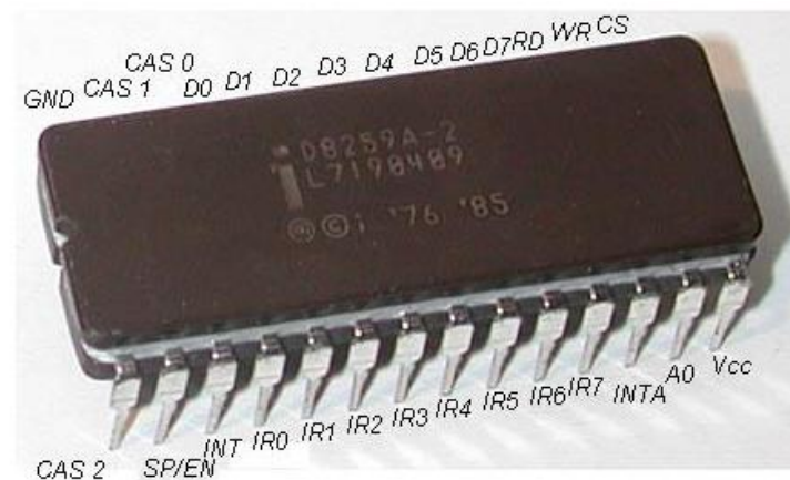
8259A PIC Microcontroller with all pins labeled.
