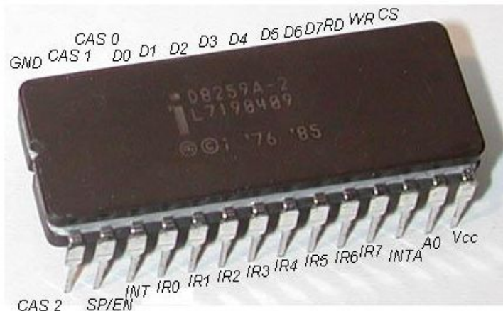
8259A PIC Microcontroller with all pins labeled.
